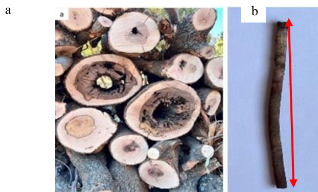
FIGURE 7. (a) Freshly felled young oak trees showing extensive fungal decay of the heartwood, resulting in complete hollowing of the trunk along a substantial portion of its height. The dark, coal-like heartwood is heavily infested with fungal growth. Photo taken in Ashkawta Village, Barzan area, on 28 October 2024. (b) Core sample extracted from an oak tree with an approximate diameter of 0.8 meters, exhibiting a black-brown discoloration and a strong odor of rot—indicative of advanced fungal degradation. Complete core extraction was unsuccessful due to advanced internal decay; the recovered core segment measured approximately 14 cm in length (red arrow) and showed pronounced fungal infestation. Photo taken in Chawrabee Village, Barzan area, on 28 January 2025.
