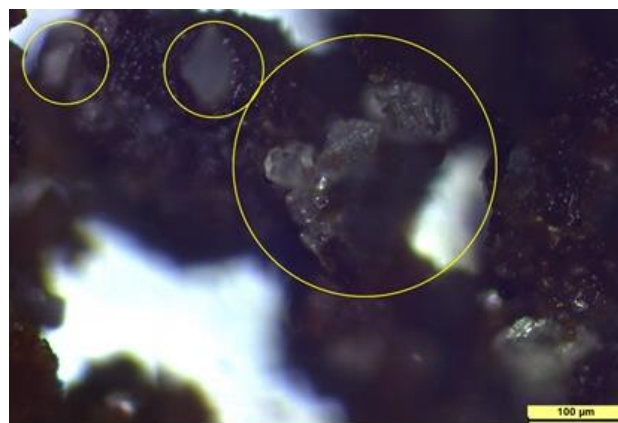
FIGURE 17B. Light microscopy images of mineral crystals extracted from decayed oak wood sample, collected in Ashkawta Village, Barzan area. Prove well-formed shape mineral oxalate crystals (yellow circle). Known to develop as metabolic by-products of fungal activity in lignocellulosic substrates, these crystalline structures fit calcium oxalate monohydrate (whewellite) and dihydrate (weddellite) morphologies [48].
